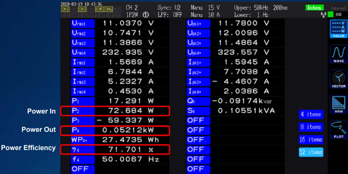
Figure 11.0 Inverter Power In, Power Out and Efficiency
